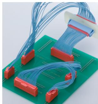
This is a 1.0mm pitch insulation displacement connector with the secure locking structure to prevent coming off the connector and incomplete mating. 1.8A in rated current was realized by using AWG#27.
