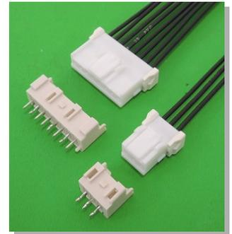
XAF connector is an insulation displacement socket connector which is compatible with the existing XA connector crimp housing (plug housing). The dipping type, SMT type, and high box type headers or the receptacle housings used for wire-to-wire connection can be prepared as the mated counterpart of XAF connector, and the wide range of connection style can be provided depending on the application.
