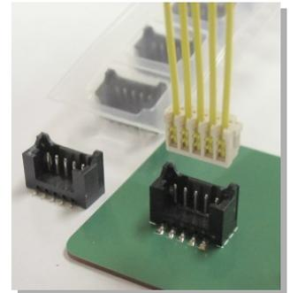
The SMT top entry type headers that can be mated with the 1.5mm pitch CZ connector socket are on the lineup.
